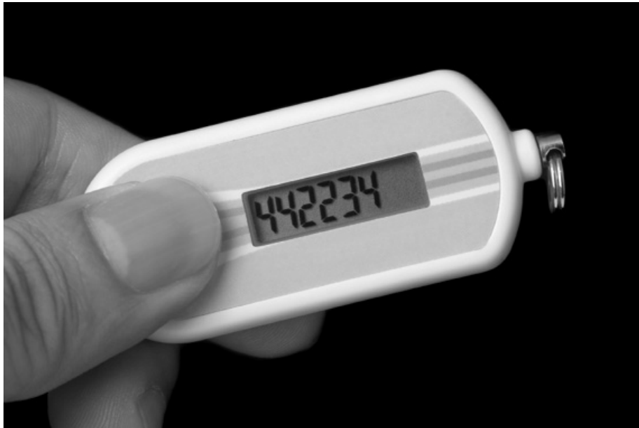
Figure 2.3: Hardware token displaying a one-time password
